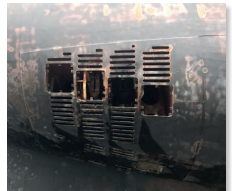
Above - Typical box cooler setup Below - External view of seachest
